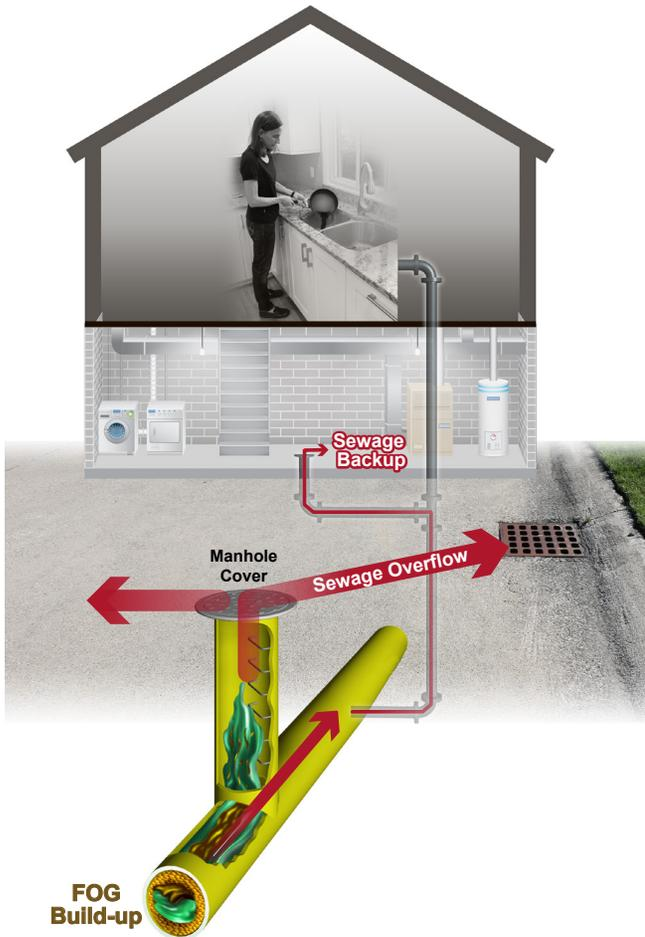
FOG enters sewer pipes through restaurant, residential and commercial sink drains. Once in the sewer, FOG sticks to the pipe and thickens. FOG can build up and eventually block the pipe and send sewage backward – out of manholes into streets and rivers, or up floor drains into homes.
